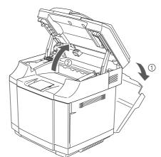
Pull out the protective part from both sides of the fusing unit.
