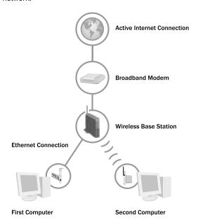
In an **ad hoc** network, a wireless adapter connects directly to wireless adapters that are installed in other computers. This type of network is often used when only two computers or devices are being connected, when a broadband Internet connection will not be shared, or when the connection to another computer is intended to be temporary. The following illustration shows an ad hoc network.
