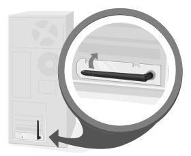
**9.** Plug in the power cord, and make sure that no other cables have come loose during installation.
