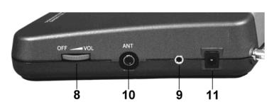
8. Off/On/Volume Control – This is the volume control and the main power switch. It lets you adjust volume to the desired listening level.
