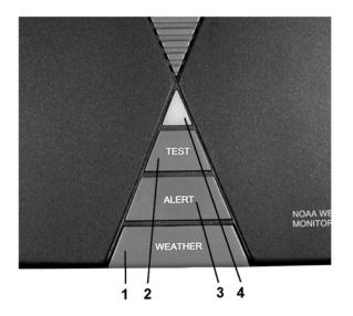
2. Alert Test Button – This is a momentary switch bar. Pressing and holding it down lets you check to see that your WR-10 tone coded alert system is operating. A loud siren-type sound will be emitted from the speaker if the ALERT switch is set to LED & ALARM.
