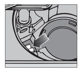
The drain pump is situated under the non-return valve (see arrow).
