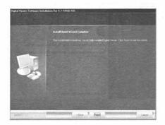
After the computer restarts, plug the microscope to the USB port of the computer. The following dialogue box will appear and the PC will automatically proceed to the hardware installation of the Digital Viewer.
