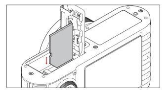
Insert the memory card (B) into the slot (1.37) with the contacts facing the battery. Push it in against the spring resistance until you hear it click into place.
