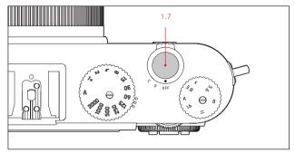
The shutter release button (1.7) works in two stages. Pressing it lightly (to the first pressure point) activates automatic focusing if set, exposure metering, and exposure control and also saves the respective settings/ values (see p. 126). If the camera was previously in stand-by mode (see p. 113), this activates the camera again and the monitor image reappears (see also p. 114). Before completely depressing the shutter release button make sure that focus-
