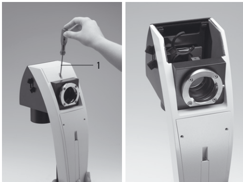
Fig. 48 Lamp housing cabling (cable duct)
