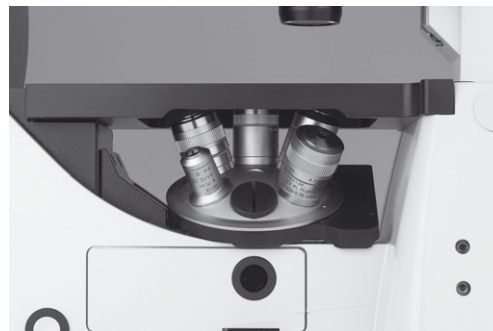
Fig. 45b Objective turret, loaded
