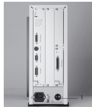
Fig. 49 Connecting the lamp housing to the Leica CTR6000 electronics box
