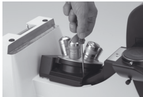
Fig. 11 Front cover, DIC prism disk
