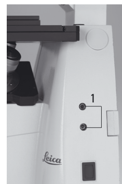
Fig. 92 Adjusting the field diaphragm (incident light-fluorescence)
