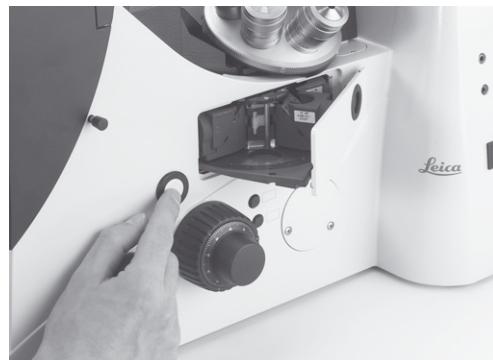
Fig. 68 Inserting or removing a filter cube
