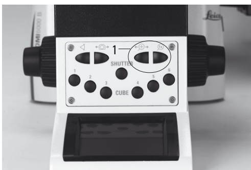
1 Function buttons for magnification changer
