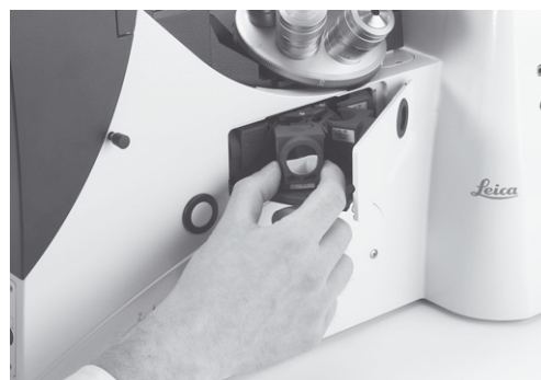
Fig. 68 Inserting or removing a filter cube
