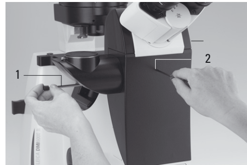
Fig. 95 Phase contrast centering procedure
