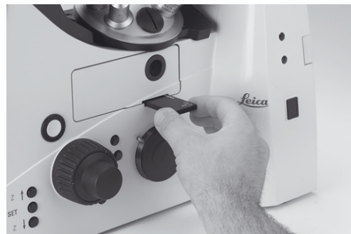
Fig. 110 Inserting the analyzer
