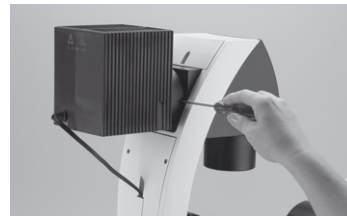
Fig. 49 Connecting the lamp housing to the Leica CTR6000 electronics box
