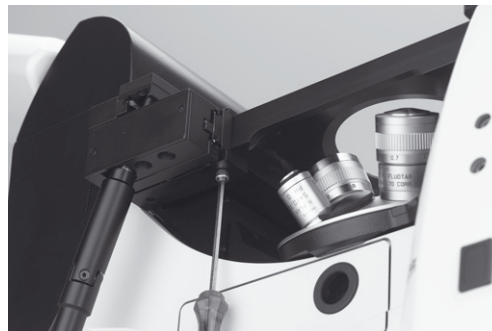
Fig. 24 Installation of attachable mechanical stage
