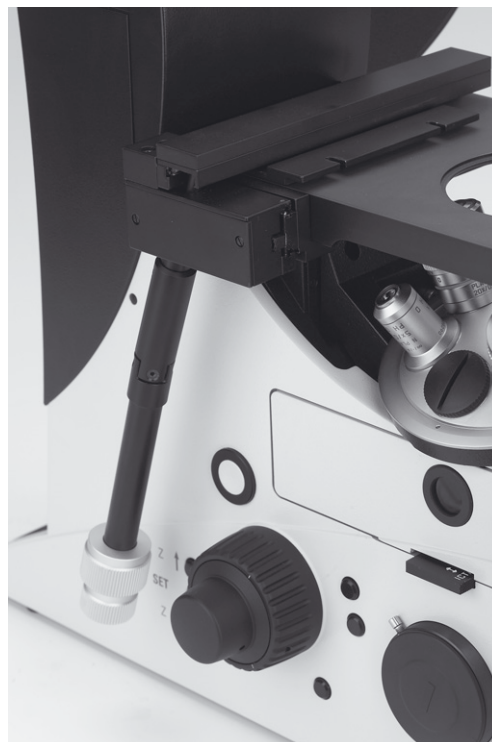
Fig. 25 Installation of attachable mechanical stage
