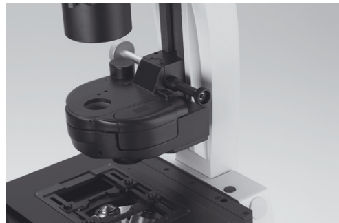
Fig. 41 Condenser on transmitted-light illumination arm
