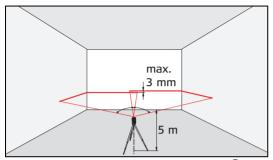
Position the instrument approx. 5 m away from the wall. Direct the instrument at the wall and switch on with the LASER key ①. Activate the laser line with the LASER key ① and mark the intersection point of laser crosshairs on the wall.
