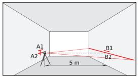
Then place the instrument at the same elevation as close as possible to wall A and again mark the horizontal laser line or the laser dot on wall A (-> A2) . Rotate the instrument by  $180^{\circ}$  again and mark the laser on wall B (-> B2). Measure the distances of the marked points A1-A2 and B1-B2. Calculate the difference of the two measurements. If the difference does not exceed 2 mm, then the Leica Lino is within tolerance.
