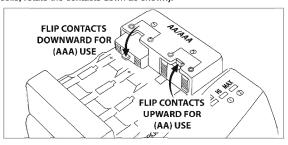
For two cells only, install both cells to be charged in position ① or position ② on the adapter plate. While the cells are being charged, the LED for position ① or position ② will glow red. Once charge is complete, the LED for that pair of cells will turn green. Remove the batteries as soon as it is practical.
