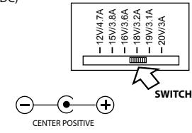
Use the diagram shown above to verify that your laptop uses "center positive" polarity as most all laptops use "center positive" polarity. Do not use the LAC90 if your laptop shows "center negative" polarity.
