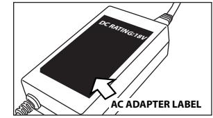
**NOTE:** The specific notation "VDC" might not be indicated. Instead the following international symbol shown might be used 18—. In some cases you may determine the desired voltage is between whole numbers such as 15.5VDC. In this case use the next higher voltage setting (16VDC)
