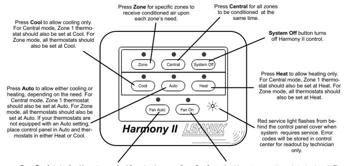
Press **Fan Auto** to allow blower to run only while system is supplying conditioned air. The blower will cycle on and off according to the demand for heating or cooling. By cycling on and off, air from different zones is not mixed and better efficiencies are achieved.
