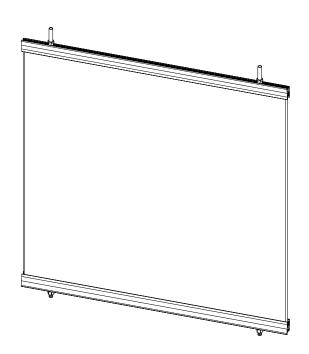
Lennox's End Panel Assembly, Models 38AEP, 38AEP-BB and 38AEP-BS are designed to be installed on Lennox's Merit Plus fireplace, Model CPF-38, along with the aluminum bi-fold glass door, Models 38ABF, 38ABF-BB and 38ABF-BS.
