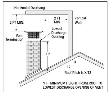
The vent/air intake termination clearances above the high side of an angled roof is as shown in the following chart:
