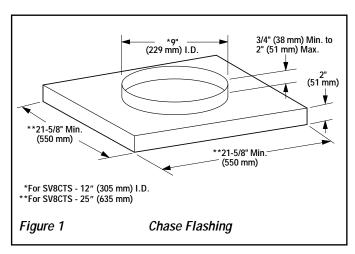
Too short of a collar or no collar at all will allow water to seep into the chase around the outside of the pipe system, and too tall of a collar will interfere with the proper attachment of the termination.
