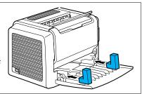
2 Replace the packing tape on the front of the original printer, and then close the media tray.
