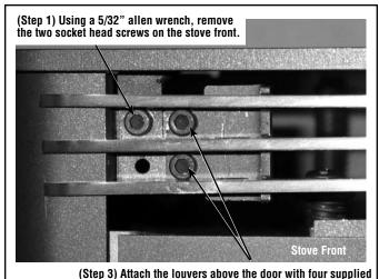
Figure 2 screws (two on left side and two on right side of stove).
