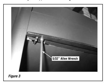
Step 3. Using a 5/32" allen wrench, attach the louvers above the door with four supplied screws (two on left side and two on right side of stove). See *Figure 1 on Page 1*.
