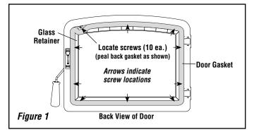
Step 3. Separate the outer door from the inner door, by pulling apart at the top, creating the necessary gap to slide the door trim in place.
