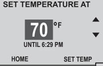
Use the UP or DOWN button to adjust to the desired temperature. This is a temporary 3-hour hold or until the next programmed event, whichever is shorter. For a longer duration see page 8.
