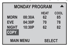
In the program screen, press the DOWN button until COPY is highlighted.
