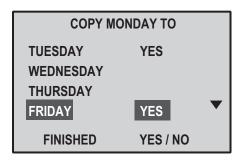
Use the UP or DOWN button to highlight the day to copy to. Press YES / NO. A YES will appear next to the day. Do this for each day to which that program is to be copied. Press FINISHED when complete.
