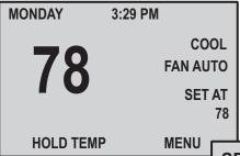
From the main screen, press the UP or DOWN button. The screen will change to the following.
