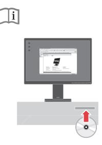
8. To optimize your monitor image, if using the analog cable, press the Automatic Image Setup key. Automatic image setup requires that the monitor is warmed up for at least 15 minutes. This is not required if you are using the DVI cable.
