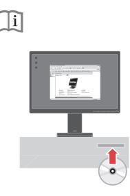
8. To optimize your monitor image, if using the analog cable, press the Automatic Image Setup key. Automatic image setup requires that the monitor is warmed up for at least 15 minutes. This is not required if you are using the DVI cable.
