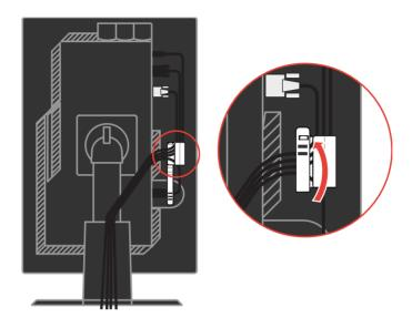
Wrap the Cable Wrapper around the cables.
