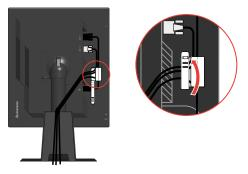
3. Wrap the Cable Wapper around the cables.
