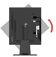
2. Place the cables(just like Power cord, VGA cable, DVI Cable) through the Main Clip. Then fasten the clip.
