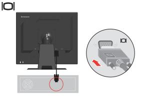
3. Connect the digital cable to the DVI connector of the monitor and the other end on the back of the computer.
