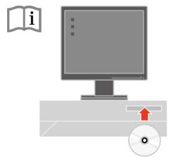
To optimize your monitor image, if using the analog cable, press the Automatic Image Setup key. Automatic image setup requires that the monitor is warmed up for at least 15 minutes. This is not required if you are using the DVI cable.
