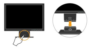
This allows access to the screws that attach the stand to the monitor.
