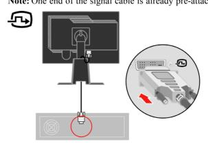
Connect the analog signal cable to the D-SUB connector of the monitor and the other end on the back of the computer.
