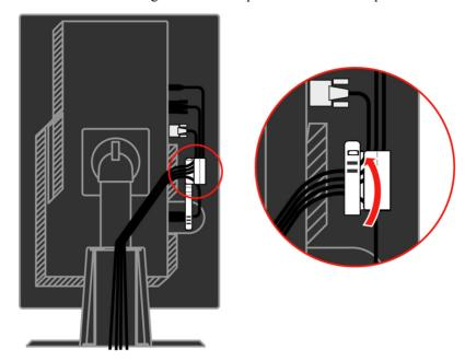
Wrap the Cable Wapper around the cables.
