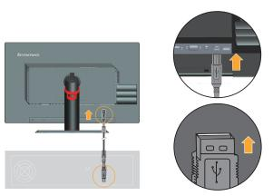
**Note:** The USB port keep available as long as the power supply is right. No matter whether the power button is on or off.
