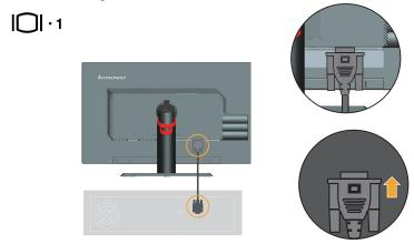
4. Connect the digital cable to the DVI connector of the monitor and the other end on the back of the computer.
