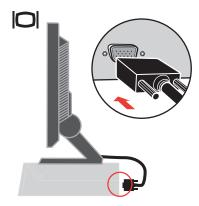
**3**. Insert the power cord into the monitor, then plug the monitor power cord and the computer cord into grounded electrical outlets.
