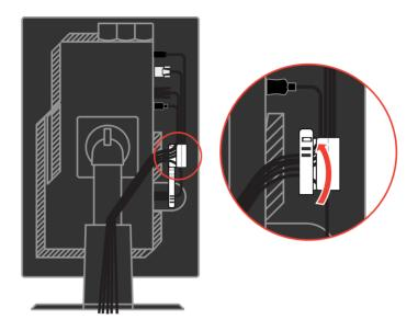
Wrap the Cable Wrapper around the cables.
