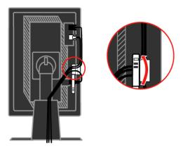
7. Wrap the Cable Wapper around the cables.
