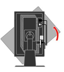
6. Place the cables through the Main Clip. Then fasten the clip.
