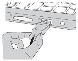
The first time you plug a USB device into a particular USB port on your computer, Windows automatically installs a driver for that device. After the driver is installed, you can disconnect and reconnect the device without performing any additional steps.
