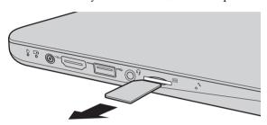
**Note:** Never insert or remove the SIM card while the computer is turned on. Doing so may cause permanent damage to the SIM card as well as the SIM card reader.
