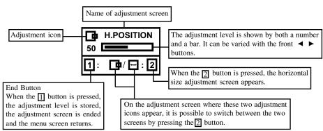
**NOTE:** The amount of adjustment depends upon how long you depress the adjustment button. You may have to tap the button to obtain the desired results.
