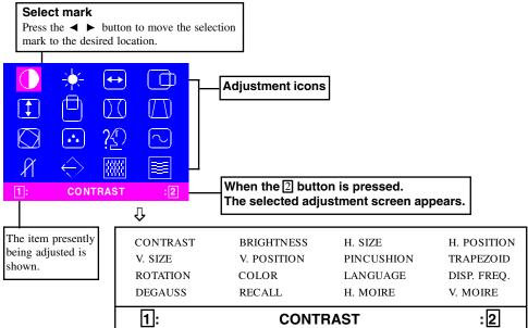
2) Adjustment screen (example: horizontal position adjustment)
