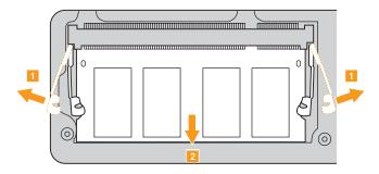
Insert the notched end of the DIMM into the socket.
