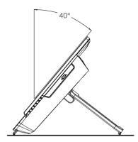
Use the stand to position the display to your preference. It can be rotated between  $15^{\circ}$  and  $40^{\circ}$  from the vertical.
