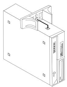
**3**. Pivot the vertical stand towards the front of the computer until it snaps into position.
