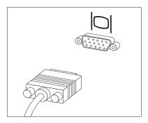
• If you have a digital video interface (DVI) monitor, your computer must have an adapter installed that supports the DVI monitor. Connect the cable to the connector as shown.
