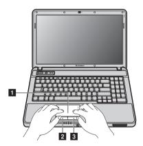
**Touchpad**To move the cursor on the screen, slide your fingertip on the pad in the direction in which you want the cursor to move.
