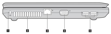
**1 Kensington slot** Attach a security lock (not supplied) here.
