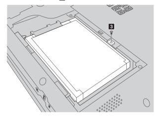
**5** Remove the frame fixing screw **3**.
