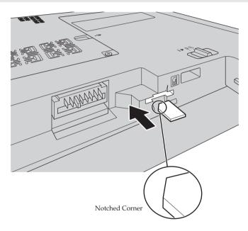
**5** Put the battery back in place. Turn the computer over and reconnect the cables.
