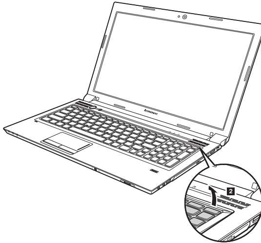
Figure 8. Removal steps of keyboard (continued)
