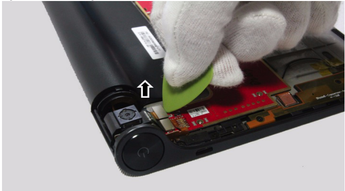
Figure 3-1 Disconnecting the main FPC
