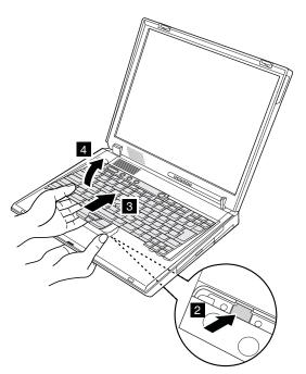
In step 2, push the keyboard from the bottom, while at the same time pushing a little in the direction of the arrow in step 3. Take care not to bend the keyboard when lifting it at step 4.
