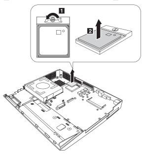
When installing: Place the CPU on the CPU socket with the pin 1 corner as shown 1, and then rotate the head of the screw in the direction of the arrow 2 to secure the CPU.
