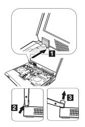
When installing: Align the hinge cover squarely and push down.
