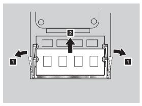
Align the notch of the DDR3 SDRAM with the protrusion of the socket and gently insert the DDR3 SDRAM into the socket at a 30-45° angle. 8 Push the DDR3 SDRAM inward toward the socket until the latches on both edges of the socket are pushed into the closed position.
