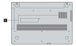
**1 Ventilation slots** Allow air to enter the computer for cooling.
