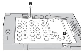
6 Take out the hard disk drive secured in a metal frame 4.
