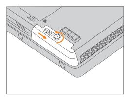
4 While holding the latch in the unlock position, remove the 2nd Hard Disk Drive.
