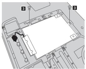
6 Carefully remove the hard disk drive (secured in the metal frame) from the compartment 4.
