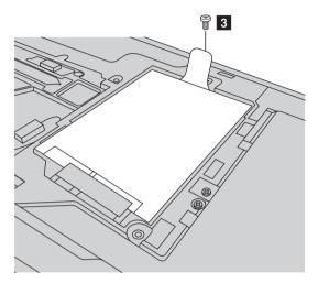
6 Pull the tab in the direction shown by arrow 4.
