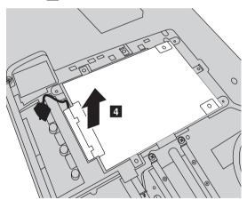
**Note:** Be sure to remove the hard disk (secured in the metal frame) gently to avoid breaking the connection to the SATA receptacle connector.
