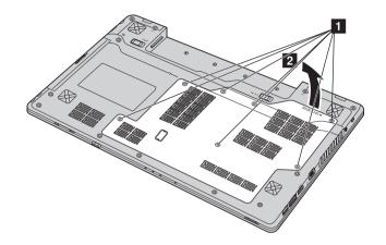
**6** Remove the frame fixing screws **3**.
