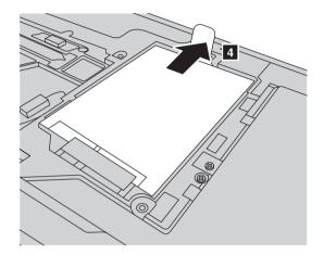
$\begin{tabular}{ll} \hline \textbf{7} & Take out the hard disk drive secured in a metal frame \\ \hline \textbf{5} & . \\ \hline \end{tabular}$
