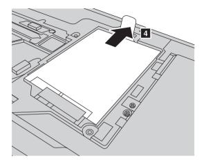
7 Take out the hard disk drive secured in a metal frame 5.
