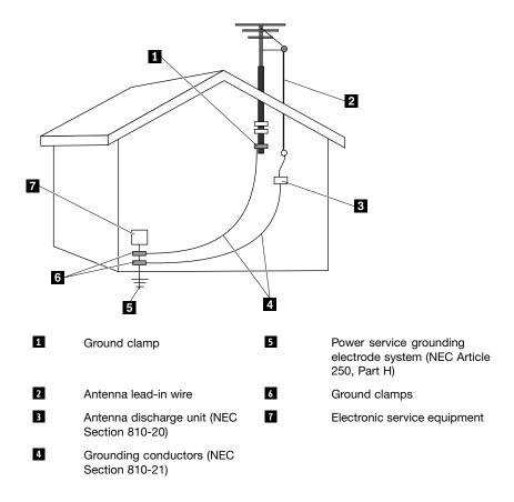
Figure 1. Proper grounding for the cable
