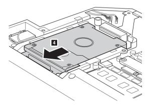
**7** Take out the hard disk drive secured in a metal frame **5**.
