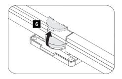
When installing: Make hinge cap parallel to LCD, and then pullup hinge to install well.
