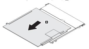
When installing: If digitizer board is defective and needs to be replaced, remove protection sheet from tape before attaching digitizer board to rear side of LCD module as shown. Tpae can be reused if there is no need to replace digitizer board.
