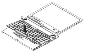
To make sure that the front side of the keyboard is housed firmly, gently press the keys with your thumbs and try to slide the keyboard toward you, shown in the step 3.
