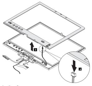
When installing: The replacement bezel should have adhesive pre-applied; therefore, remove the covering from the bezel to expose the adhesive, and then place the top edge under the frame, shown as 1, then push the bezel down and secure with the latches firmly. Be careful not to make the bezel touch the Bluetooth antenna from being deformed downward or inward as B . Make sure Bluetooth antenna is not deformed as A.
