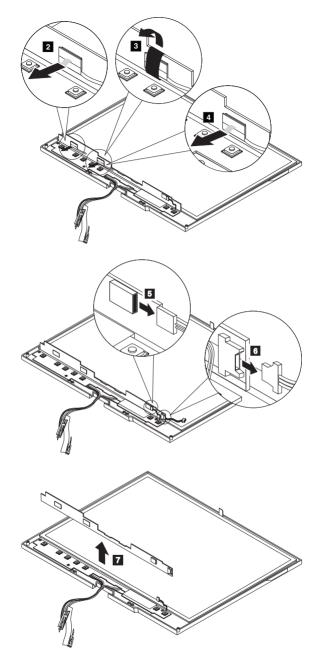
When installing: Make sure that all the connectors attached firmly.
