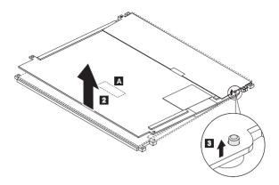
Note: One piece of tape, indicated as A, sticks between digitizer board and LCD module. Be careful to remove digitizer board slowly in step 2.
