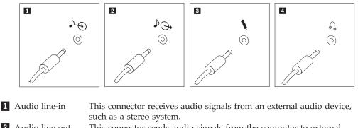
2 Audio line-out This connector sends audio signals from the computer to external devices, such as powered stereo speakers.
