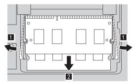
Align the notch of the DDR3 SDRAM with the protrusion of the socket and gently insert the DDR3 SDRAM into the socket at a 30-45° angle.
