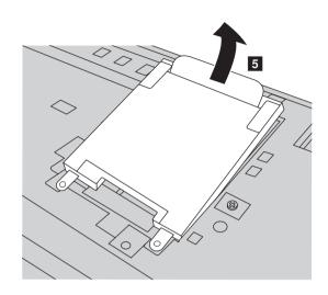
Take out the hard disk drive secured in a metal frame 5.Lenovo IdeaPad Z380
