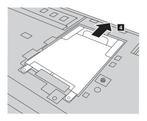
6 Pull the tab in the direction shown by arrow 4.Lenovo IdeaPad Z380
