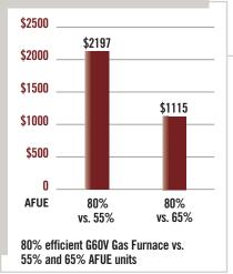
This chart depicts potential energy savings you can expect from the G60V furnace, versus older furnaces with lower efficiency ratings. Criteria used in this example are 2,000 full-load heating hours, with a 60,000 Btuh heating design load and \$1.074 ccf for gas. Your actual savings may vary, depending on the weather patterns in your local area, local fuel rates and your individual lifestyle. Source: U.S. Environmental Protection Agency (EPA) national average energy rates.
